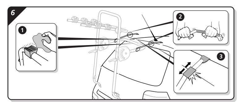
(1) Before offering the carrier to your vehicle ensure the rear window/bodywork and rubber feet on the vehicle support arm are clean and free of dust. (2) For most vehicles it will be necessary to pre-bend the plain flat section of the metal straps. (3) Offer the carrier
